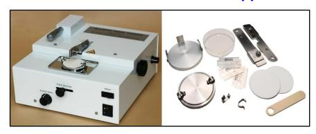
This apparatus has been designed to prepare pieces of tissue for metabolic experiments and is especially suitable for small and irregular specimens available at biopsy or from small organs. It causes much less disturbance to cell structure than homogenisers or blenders and is applicable to fragments that would be difficult or impossible to cut by ordinary methods. Typical applications are to liver, kidney and various parts of the central nervous system.
