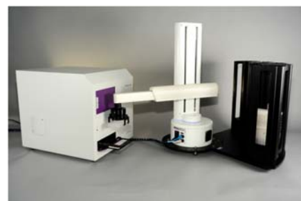
SciClops™ with plate rack delivering plates to an instrument
