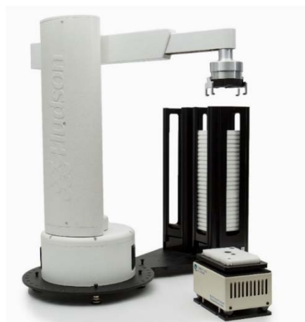
SciClops™ with standard and temperature controlled racks
