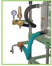
SS inlet / outlet adapters, available in M16 x 1 and M30 x 1.5, allow connection to cooling / heating circulator
