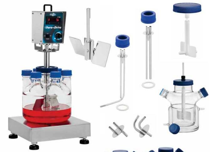
**Bioreactor Vessels** with four or six vertical side arms. Available from 3 to 36 liters, in high or low profile form.
